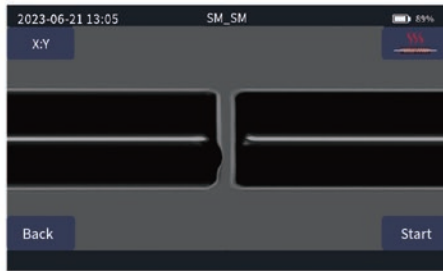
Uneven end face of optical fiber
